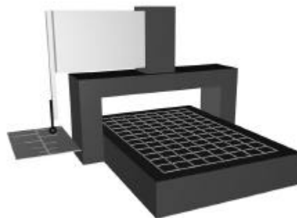
Figure 3. Scanning the LPDA using the coordinate table.
